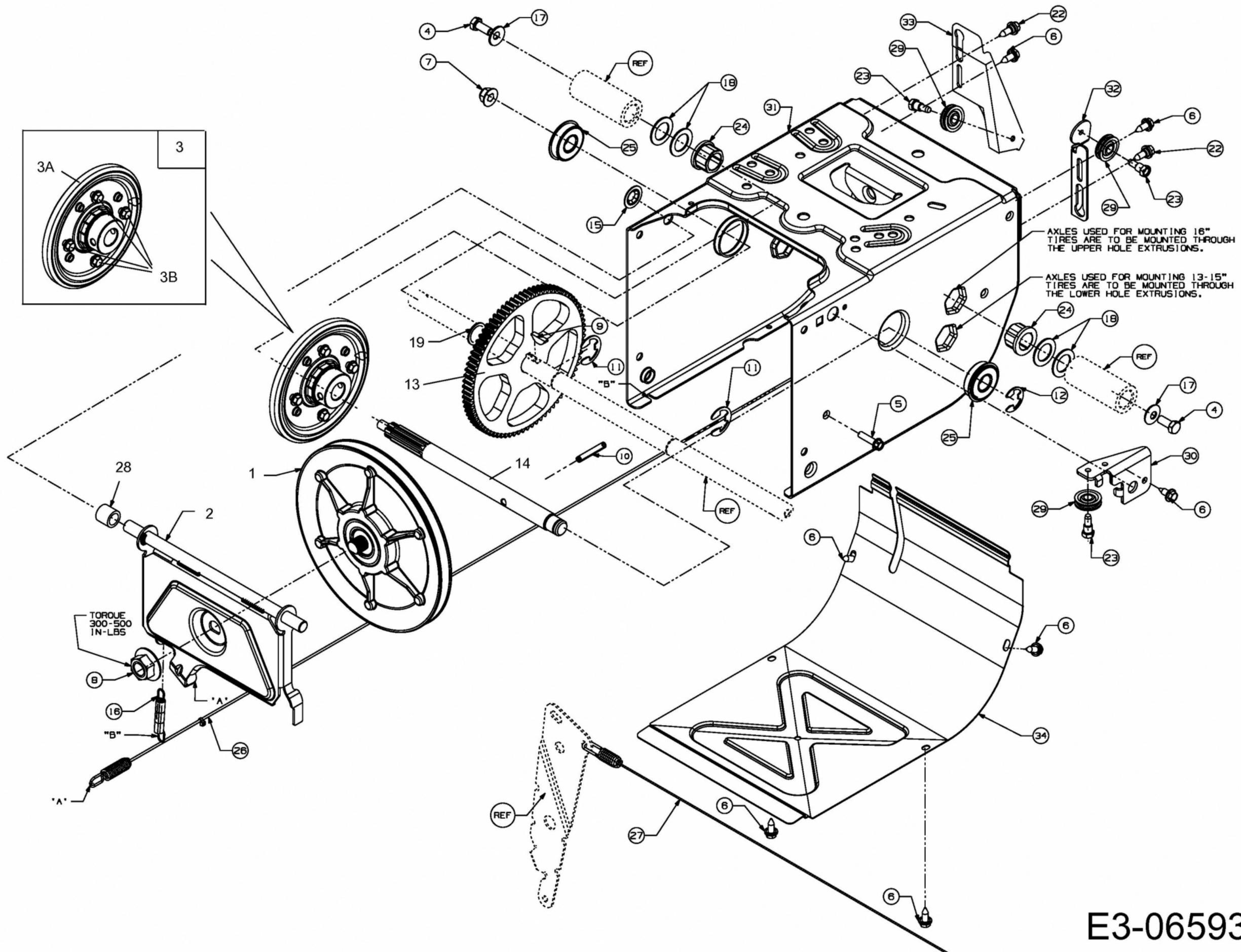
AXLES USED FOR MOUNTING 16" TIRES ARE TO BE MOUNTED THROUGH THE UPPER HOLE EXTRUSIONS.
